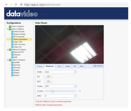
The exposure option allows users to set Exposure Mode, EV, BLC, Anti-Flicker, Gain Limit and DRC.
