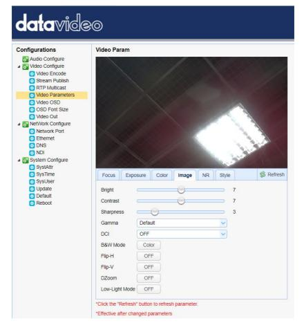
The Image option allows users to set several parameters including Bright, Contrast, Sharpness, Gamma, DCI, B & W Mode, Flip-H, Flip-V and DZoom.
