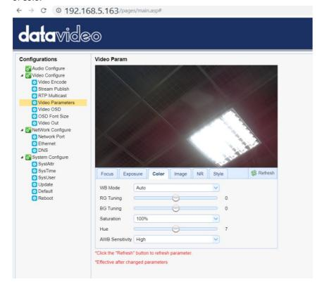
The Color option allows user s to set WB Mode, RG Tuning, BG Tuning, Saturation, Hue and AWB Sensitivity.
