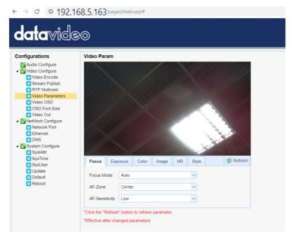
Focus Option provides users to set Focus Mode, AF-Zone and AF-Sensitivity. Focus Mode: Users can select Auto, Manual and One Push from the drop down menu.
