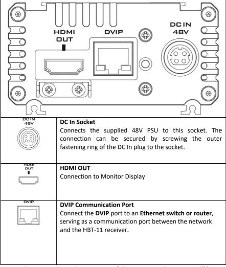
Note: The HBT-11 is not the accessory of the PTC-140T, The HBT-11 will be packaged only with the PTC-140TH.
