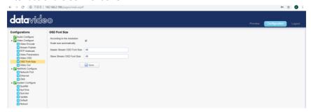
Please check the checkbox of "According to the resolution" "Scale Size automatically" and then the font size will be scaled automatically. Moreover, users can enter their desired font size into the blanks of "Master Stream OSD Font Size" and "Slave Stream OSD Font Size" and then please click the "Save" button to apply the font size.
