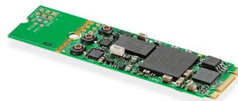
Miniature M.2 card with 3G-SDI connections for simultaneous capture and playback in all SD and HD formats up to 1080p60. DeckLink SDI Micro also includes Black Burst and Tri-Sync reference input and its miniature size makes it great for use on portable solutions which are based on compact computers!
