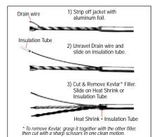
Terminating L-4E5AT and L-4E6AT (Foil Shield)
