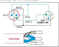
Because the shield density on Canare Cable is very high, it is somewhat difficult to push back the braid and pull the inner conductors through. Instead, we strongly recommend unbraiding the shield by "combing" it out with a pointed tool, beginning at the end of the cable.
