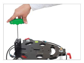
• Fix Wedge Tilt Plate onto base plate and tighten the allen screw.
