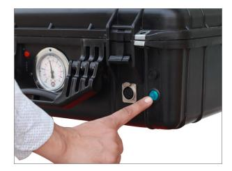
You can check Battery level by switching on the Battery Status Indicator button. If it is low, then you need to get it charged at the earliest. It connects to socket and also directly to car for charging (both cables included).
