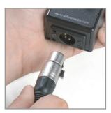
To power the Controller you must insert the 4-pin XLR connector from the Power Supply. A camera battery can also be used to power the unit.
