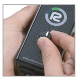
The intensity of the LiteRing can be changed using the dial on the Controller. - 5 is the lowest setting on the Controller and +5 is the highest.
