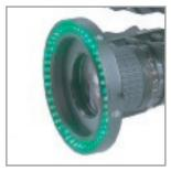
Once the LiteRing is securely fastened to the lens it should not move.
