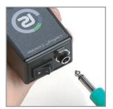
Inset the 1/4 inch jack from the LiteRing into the Contrroller. To turn the unit on, use the the on/off switch. The Controller will illuminate once powered.
