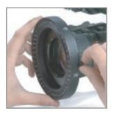
Place the LiteRing over the top of the adapter and tighten the metal screw.
